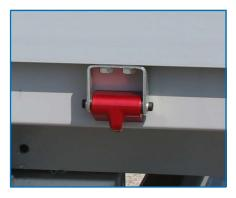
Standard side-panel pivoting system with hook for ropes.
