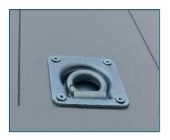
Eyelets certified according to DIN EN 12640 norm.
