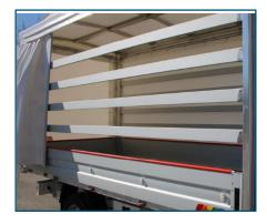
Removable curtainsider structure made of aluminium light alloy, available as OPT.
