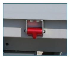
Standard side-panel pivoting system with hook for ropes.
