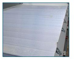
Aluminium loading floor with smooth or anti-skid surface, ideal for concentrated loads and corrosive substances, available as OPT.
