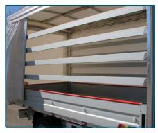
Removable curtainsider structure made of aluminium light alloy, available as OPT.
