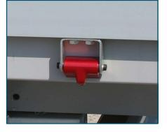
Standard side-panel pivoting system with hook for ropes.
