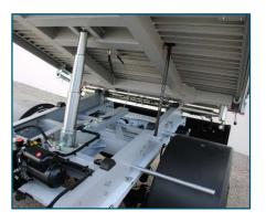
Tipper and subframe entirely made of structural aluminium alloy.
